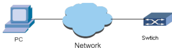
Figure 1-14. TFTP configuration diagram.
